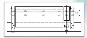
**6. Wind deflector brush**, in the aluminum profile AN 5/25 — intended for hermetically sealed connection of wind protection to the roof. It prevents snow from blowing in and loss of pressure difference, which increases the efficiency of the exhaust system by at least 10%.
